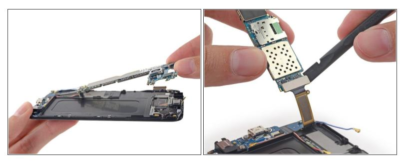
• The motherboard is still held by the gravitational pull of a pesky daughterboard connector. We quickly set to work with a spudger and lift off to get a closer look.
