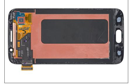
With the display removed, we find the same <u>STMicro FT6BH</u> <u>touchscreen controller</u> as the [invalid guide link].
