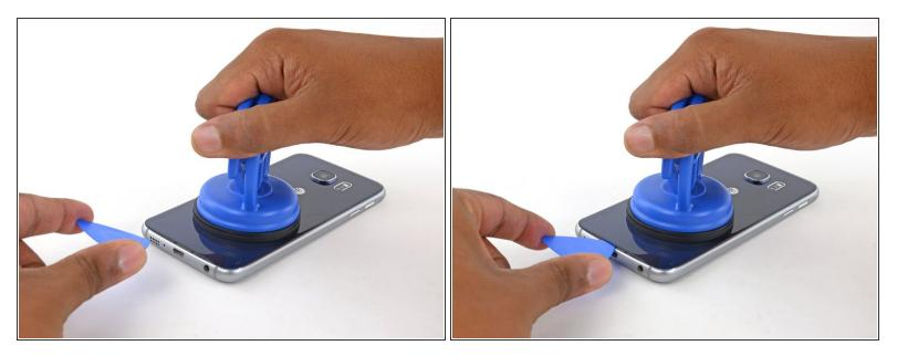
Once you've opened a large enough gap, insert an opening pick between the rear glass and the midframe.
