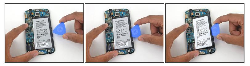
Insert a plastic opening pick between the case and the battery.
