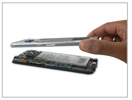
Lift the midframe assembly up to separate it from the rest of the phone.
