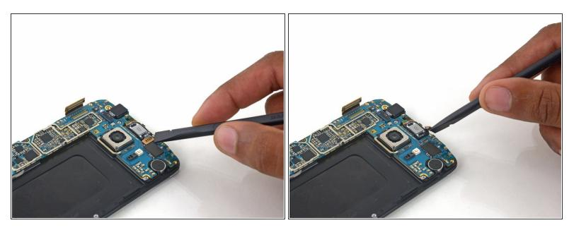
Disconnect the earpiece speaker assembly cable connector from the motherboard.
