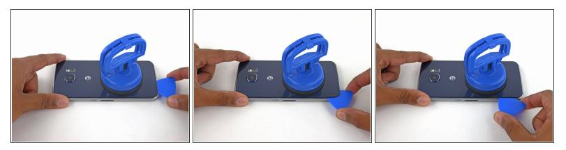
• Slide the opening pick around the bottom left corner of the rear glass panel.
