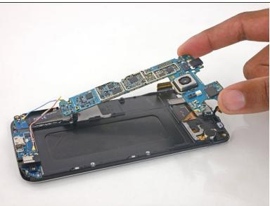
Lift the camera-side end of the motherboard to separate it from the display frame.
