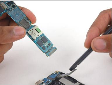
Disconnect the daughterboard ribbon cable connector from its socket on the underside of the motherboard.
