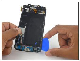
Slide the pick downwards to separate the display frame from the display assembly.
