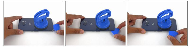
Slide the opening pick around the bottom left corner of the rear glass panel.
