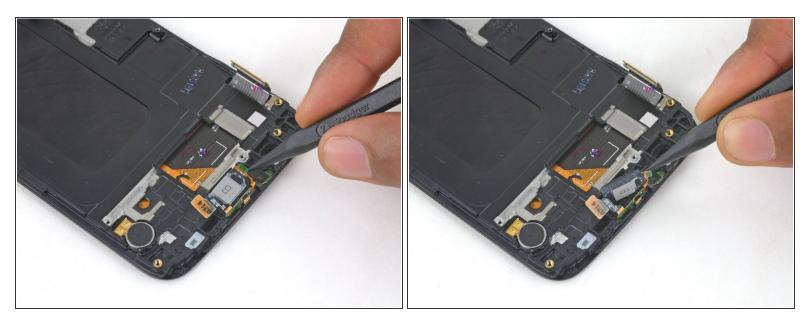
• Use the pointed edge of the spudger to lift the earpiece speaker assembly from the display frame.
