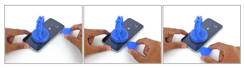
Slide the opening pick down along the volume buttons side of the phone.
