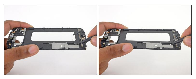
• Use the pointed end of a spudger to push the home button cable through the display frame.
