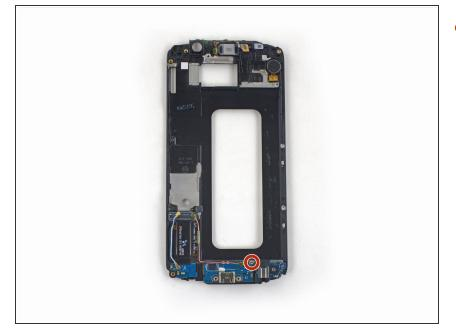
Remove the single 3.0mm Phillips #00 screw securing the daughterboard to the display frame.
