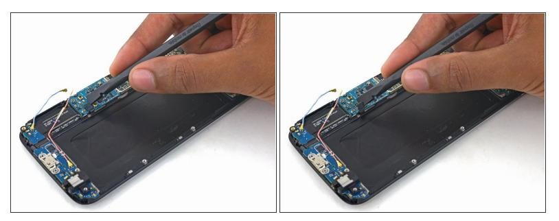
• Use the flat end of the spudger to disconnect the home button connector.
