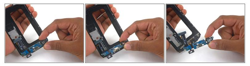
(i) Flip the frame over again and lift up the daughterboard to peel it off the display frame.
