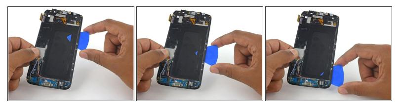
• Slide the pick downwards to separate the display frame from the display assembly.
