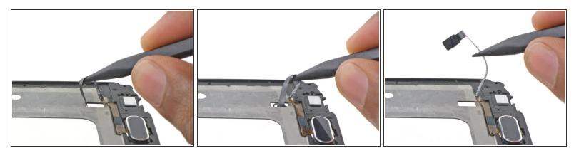
• Flip the display frame over and use the pointed end of a spudger to pull the home button cable completely through the hole.
