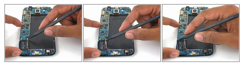
• Use the pointed edge of a spudger to disconnect the Bluetooth and Wi-Fi antenna cable connectors from their sockets on the motherboard.
