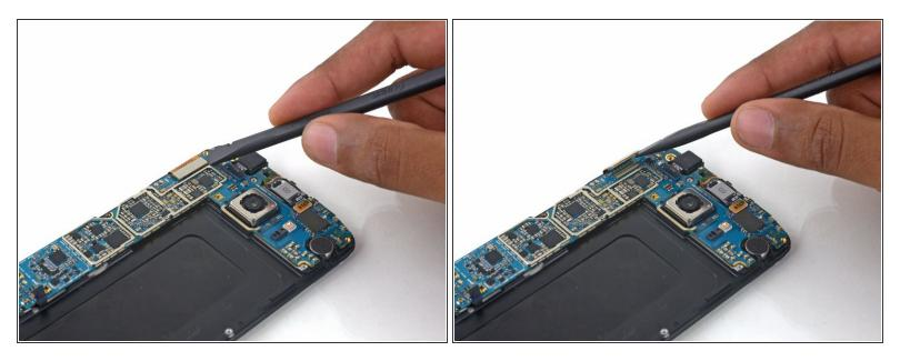
• Use the flat end of a spudger to disconnect the display assembly cable from the motherboard.
