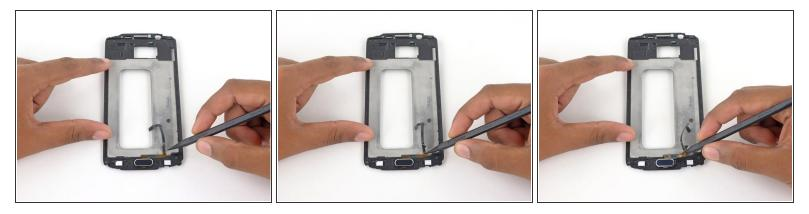
• Slide the spudger under the cable to continue separating it from the frame.
