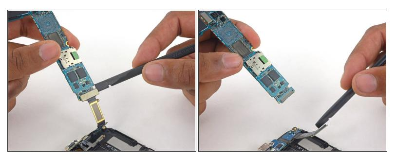
Disconnect the daughterboard ribbon cable connector from its socket on the underside of the motherboard.
