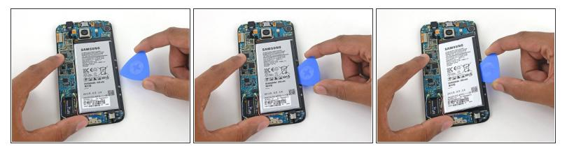
Insert a plastic opening pick between the case and the battery.
