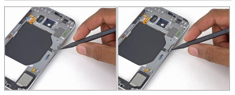
Use the pointed end of the spudger to push the power button out of the midframe.
