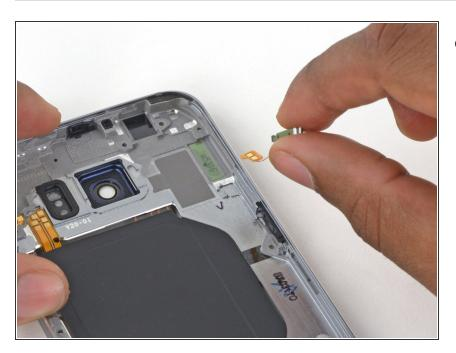
Remove the power button bracket assembly.
