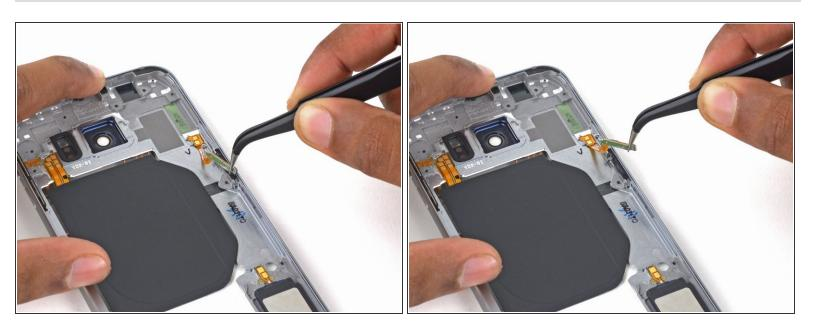
Pull up lightly on the power button ribbon cable until only the the spring contacts are still adhered to the midframe.
