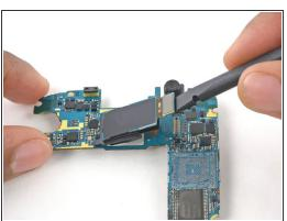
Use the flat end of a spudger to disconnect the rear-facing camera connector from its socket on the motherboard.
