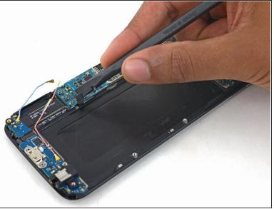
Use the flat end of the spudger to disconnect the home button connector.
