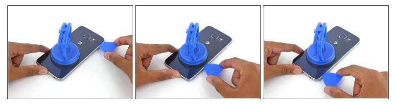
• Slide the opening pick down along the volume buttons side of the phone.
