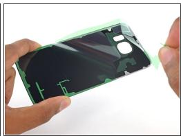
Peel back the inner film layer.
