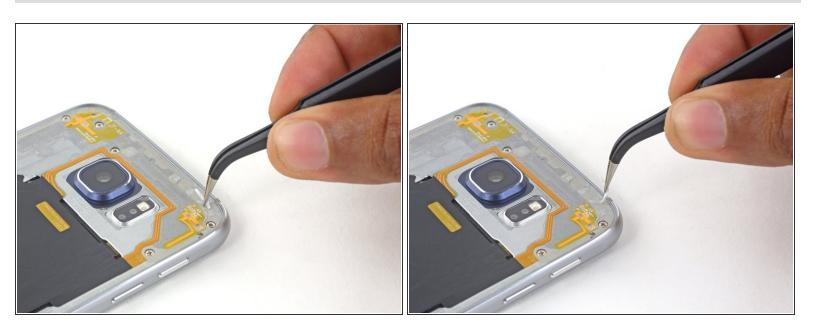
Use a pair of tweezers to remove any adhesive still on the midframe.
