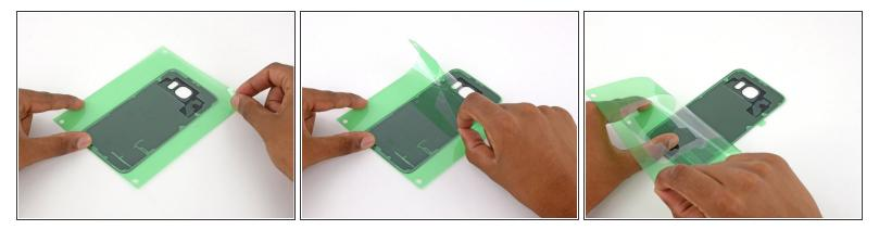
Peel back the outer layer of green film.
