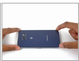
• Lower the rest of the rear panel and press it firmly into the midframe.
