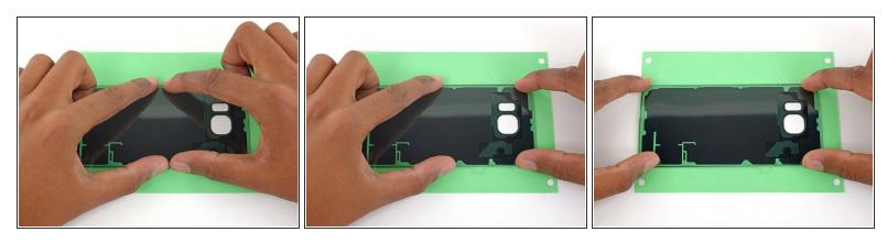
Run your fingers over the tape to firmly attach it to the glass.
