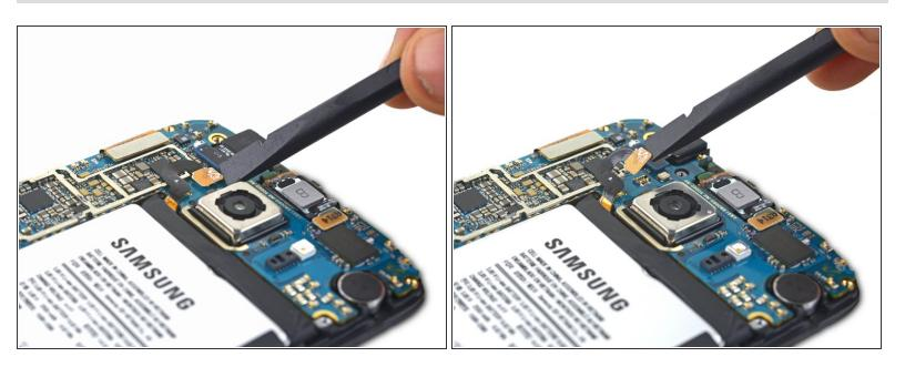
Use the flat end of the spudger to disconnect the battery connector from its socket on the motherboard.
