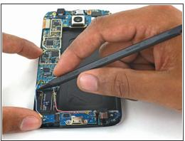
Use the pointed edge of a spudger to disconnect the Bluetooth and Wi-Fi antenna cable connectors from their sockets on the motherboard.
