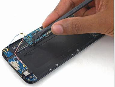
Use the flat end of the spudger to disconnect the home button connector.
