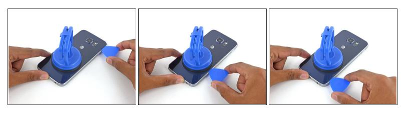
Slide the opening pick down along the volume buttons side of the phone.
