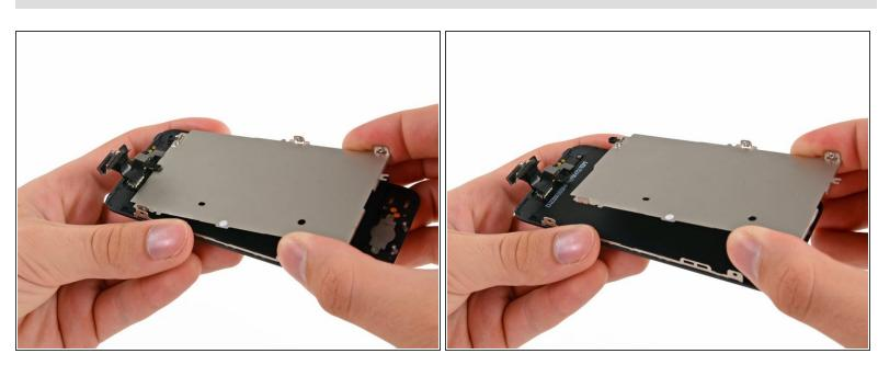
Remove the LCD shield plate from the display assembly.
