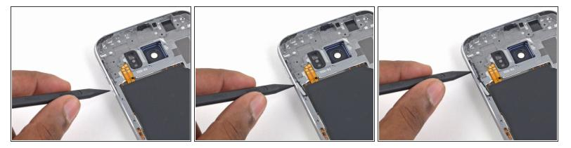
Use the pointed end of the spudger to push the button covers out of the midframe.
