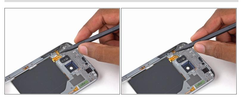
Use the pointed end of the spudger to pry up the volume button contact connectors.
