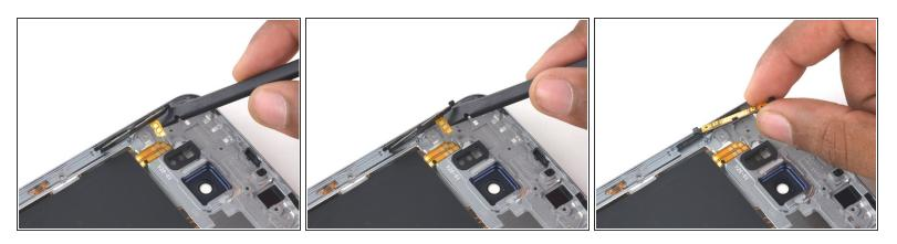
• Use the flat end of the spudger to pry the volume buttons out of the midframe.
