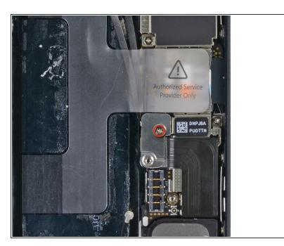
Remove the single 1.2 mm Phillips screw remaining in the mid-section logic board bracket.
