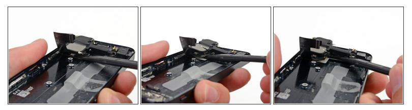
• Use the flat end of a spudger to gently pry the Lightning connector and speaker enclosure assembly cables up from the rear case.
