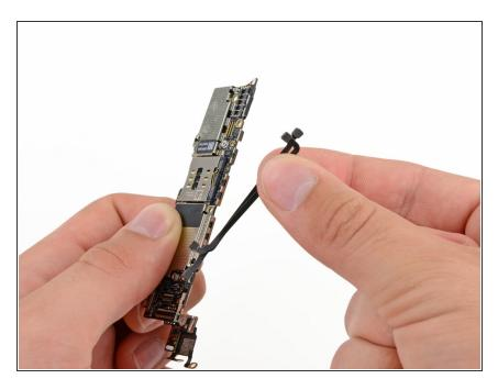
Remove the two interconnect cables from the logic board.
