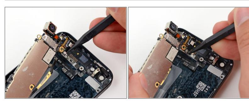
Use the tip of a spudger to pry the Wi-Fi antenna cable connector up from its socket on the underside of the logic board.
