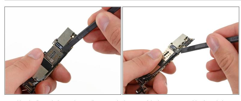
Use the flat end of a spudger to disconnect the bottoms of the interconnect cables from their sockets on the logic board.
