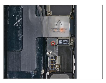
Remove the single 1.2 mm Phillips screw remaining in the mid-section logic board bracket.
