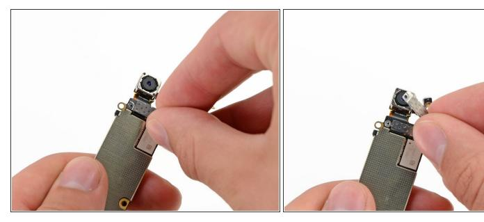
Remove the rear-facing camera bracket from the logic board.
