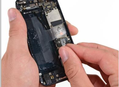
Remove the mid-section bracket from the logic board.
