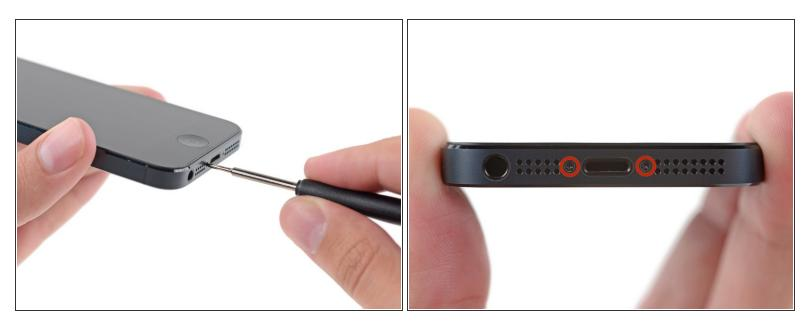
Insert the two 3.6 mm Phillips screws into the screw holes using the provided #000 Phillips screwdriver.
