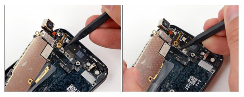
Use the tip of a spudger to pry the Wi-Fi antenna cable connector up from its socket on the underside of the logic board.
