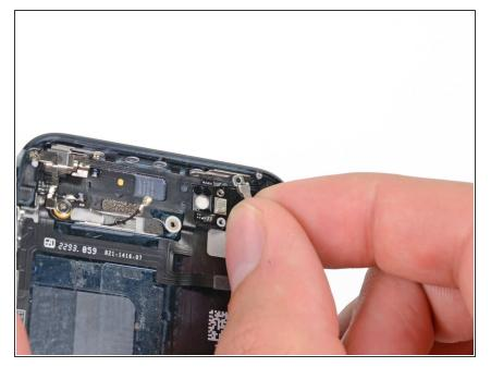
Remove the metal bracket between the rear facing flash and camera windows.
