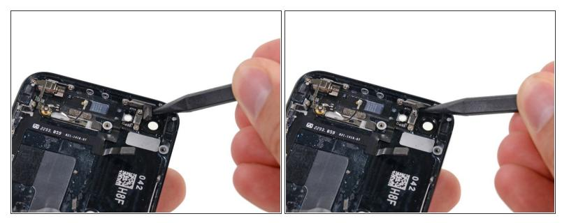
• Use the tip of a spudger to remove the rubber bumper from below the power button.
