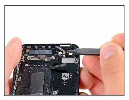
Use the tip of a spudger to press the power button cover in and lift it off of its hinge in the rear case.
