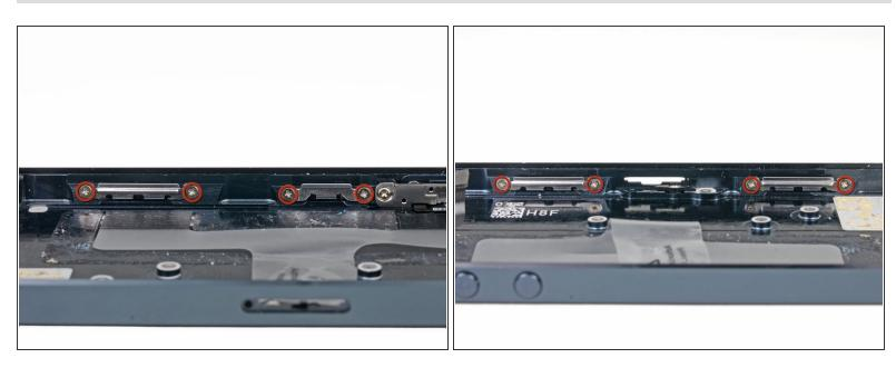
Remove eight 1.3 mm Phillips screws securing the front panel clips to the interior sides of the rear case.
