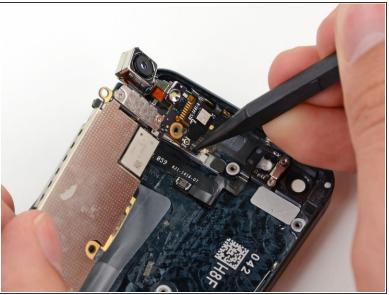
Use the tip of a spudger to pry the Wi-Fi antenna cable connector up from its socket on the underside of the logic board.
