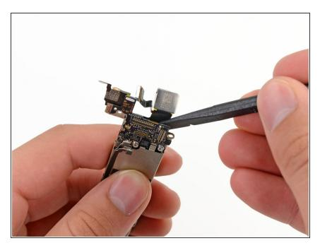
Use the flat end of a spudger to disconnect the rear-facing camera cable from its socket on the logic board.
