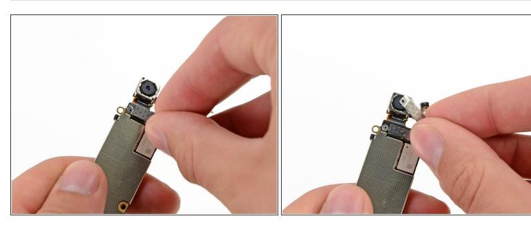
Remove the rear-facing camera bracket from the logic board.
