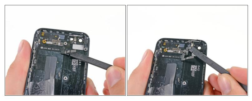
• Use the flat edge of a spudger to pry the cable up from the adhesive securing it to the rear case.
