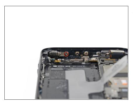
Remove the 1.6 mm Phillips screw securing the vibrator to the top inside of the rear case.
