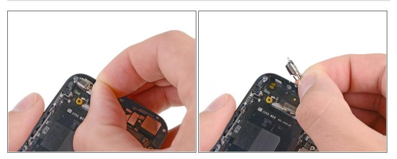
Remove the vibrator from the rear case.
