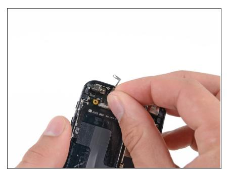
Remove the vibrator bracket from the rear case.
