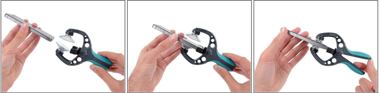
**i** The next two steps demonstrate using the [iSclack](#), a great tool for safely opening the iPhone 5 that we recommend for anyone doing more than one repair. **If you aren't using the iSclack, skip to [\[invalid guide link\]](#).**
