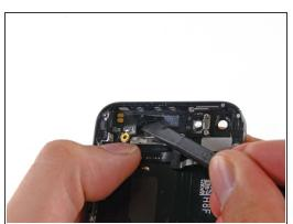
Starting under the cable connection, use the flat of a spudger to pry the Wi-Fi antenna up from the rear case.
