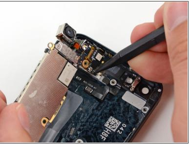
Use the tip of a spudger to pry the Wi-Fi antenna cable connector up from its socket on the underside of the logic board.
