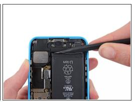
Run the tip of a spudger between the battery and the headphone jack to unfold the battery adhesive tab.
