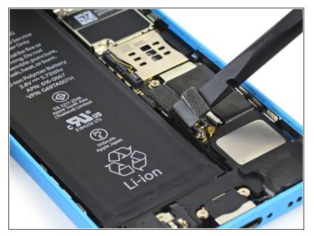
• Use the flat edge of a spudger to pry the battery connector up off the logic board.
