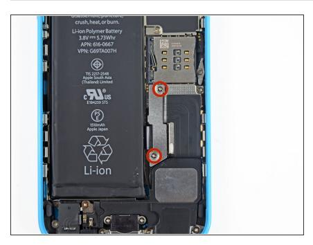
Remove the two 1.6 mm Phillips #000 screws securing the metal battery connector bracket to the logic board.
