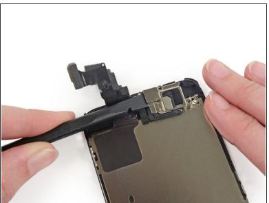
Use the flat edge of a spudger to push the earpiece speaker bracket off the display assembly.
