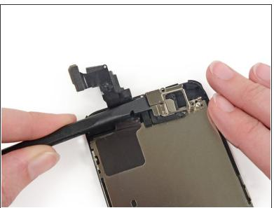
Use the flat edge of a spudger to push the earpiece speaker bracket off the display assembly.
