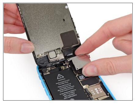
• Remove the front panel assembly cable bracket from the logic board.
