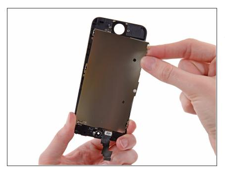
• Remove the LCD shield plate from the display assembly.
