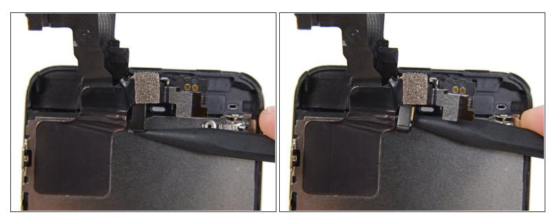
• Slide the point of a spudger under the microphone to lift it out of its recess in the display assembly.
