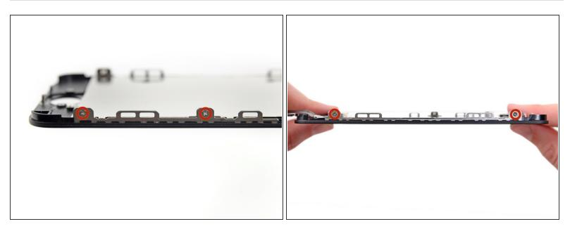
Remove two 1.2 mm Phillips #000 screws from each side of the LCD frame (four total).
