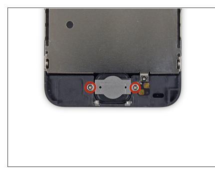
Remove the two 1.3 mm Phillips #000 screws securing the home button bracket to the display assembly.
