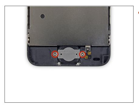
Remove the two 1.3 mm Phillips #000 screws securing the home button bracket to the display assembly.
