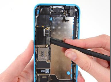
The Lightning connector cable is lightly adhered to a shield on the logic board. Use the flat end of a spudger to gently peel the cable up.
