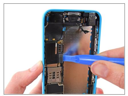
Use a plastic opening tool to disconnect the Lightning connector ribbon cable from its socket on the logic board.
