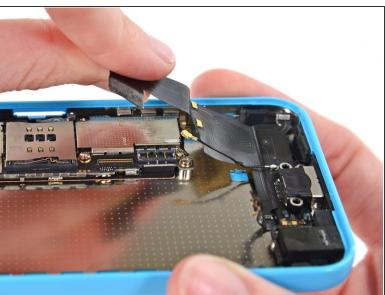
Gently peel the Lightning connector assembly up from the rear case.
