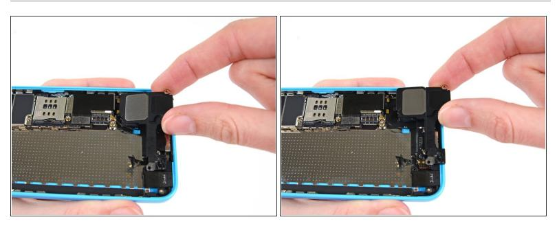
Remove the speaker enclosure. Be careful not to snag it on the antenna cable.
