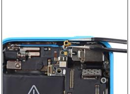
Pull the logic board away from the rear-facing camera just enough to expose the gold contact cap under the top end of the board.
