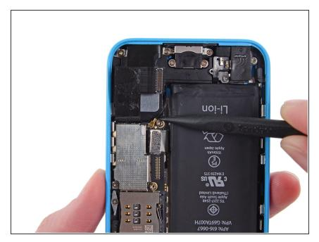
Disconnect the antenna connector from the base of the logic board.
