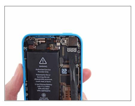
Disconnect the rear facing camera cable connector from its socket on the logic board.
