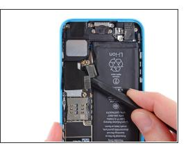
The Lightning connector cable is lightly adhered to a shield on the logic board. Use the flat end of a spudger to gently peel the cable up.
