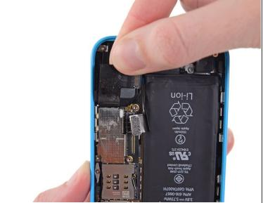
Fold the cable up out of the way of the logic board.
