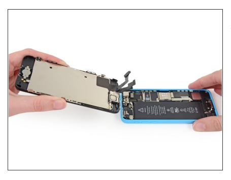
Remove the front panel assembly from the rear case.
