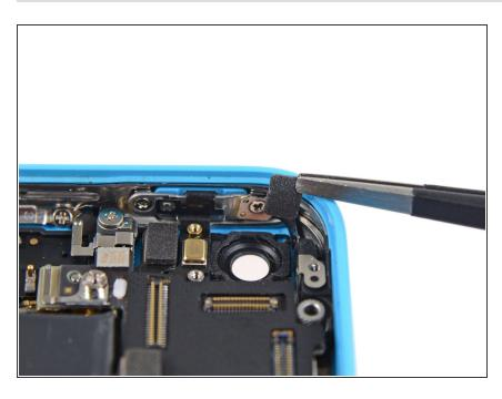
Remove the small foam tape from inside the rear camera's cavity.
