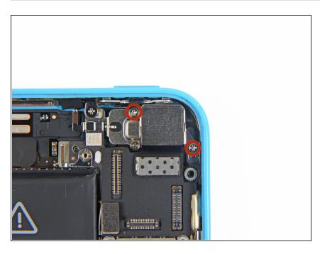
Remove the two 1.5 mm Phillips #000 screws securing the rearfacing camera to the rear case.
