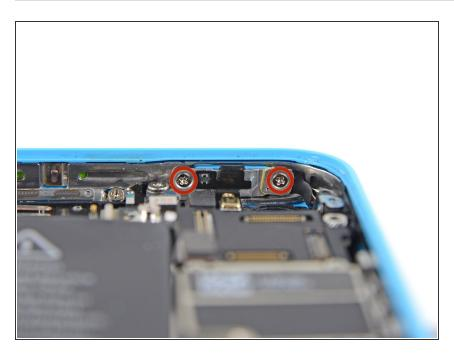
Remove the two 1.4 mm Phillips #000 screws securing the power/sleep button bracket.
