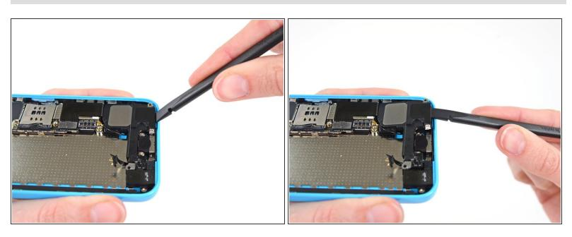
• Use the flat end of a spudger to gently pry the speaker enclosure up from the rear case.
