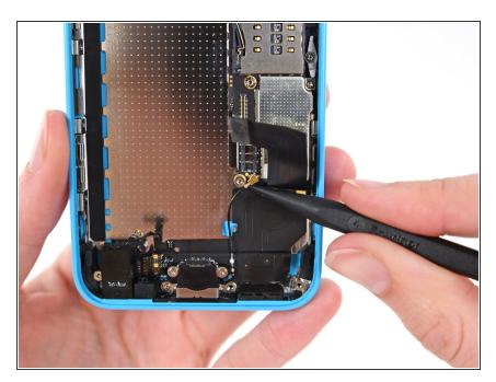
Disconnect the cellular antenna connector from the base of the logic board.
