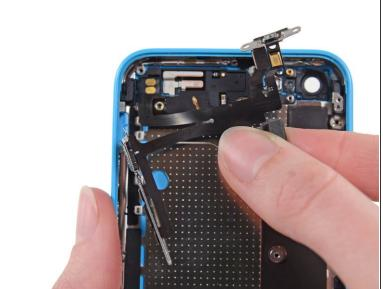
Peel the upper assembly cable up from right to left to separate the adhesive holding it to the case.
