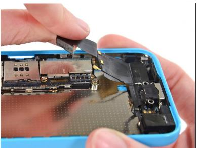
Gently peel the Lightning connector assembly up from the rear case.
