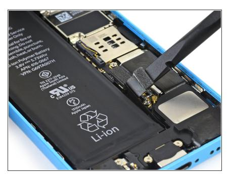
Use the flat edge of a spudger to pry the battery connector up off the logic board.
