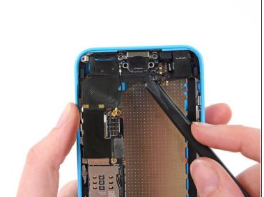
You may need to use the flat end of a spudger to completely free the assembly.
