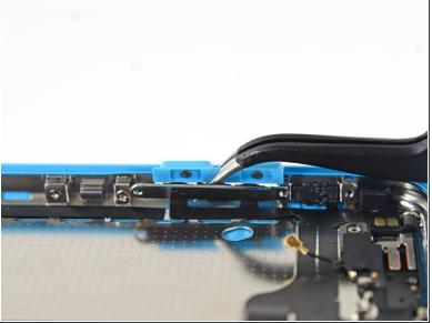
• Use the tip of a spudger to fold the volume rocker bracket down from the side wall. Remove the volume rocker.
