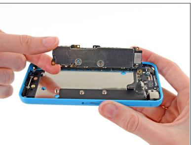
Flip the logic board up toward the volume control buttons to expose the antenna connector.
