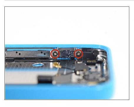
Remove the two 1.6 mm Phillips #000 screws from the hold switch bracket.
