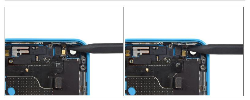
Use the tip of a spudger to peel the power/sleep button cable off of the rear case.
