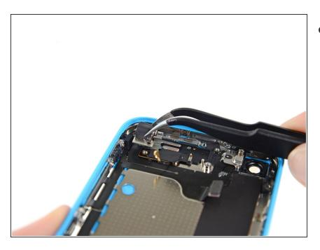
Remove the vibrator motor.
