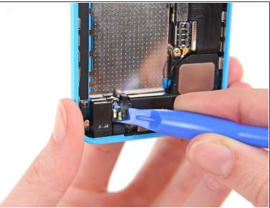
Use a plastic opening tool to peel the home button spring contact cable up from the speaker enclosure.
