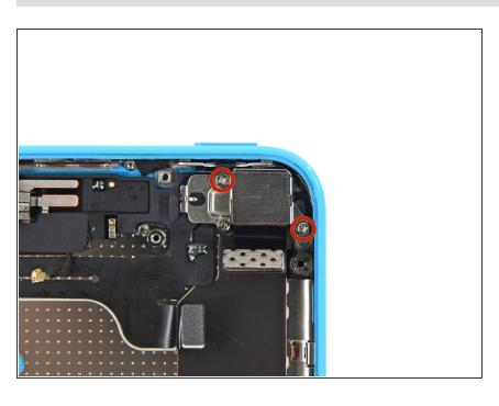
Remove the two 1.5 mm Phillips #000 screws securing the rear camera cover to the rear case.
