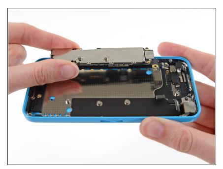
Remove the logic board from the rear case.
