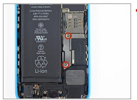
Remove the two 1.6 mm Phillips #000 screws securing the metal battery connector bracket to the logic board.
