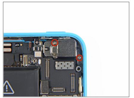
Remove the two 1.5 mm Phillips #000 screws securing the rearfacing camera to the rear case.
