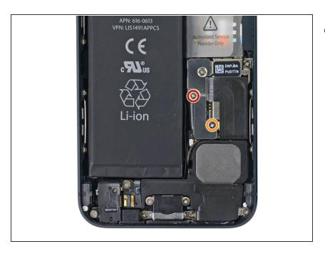
Remove the following two screws securing the metal battery connector bracket to the logic board:
