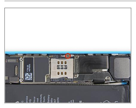
Remove the 2.0 mm Phillips #000 screw securing the SIM ejector.
