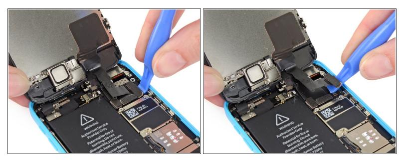
• Use a plastic opening tool to disconnect the front-facing camera and sensor cable connector.
