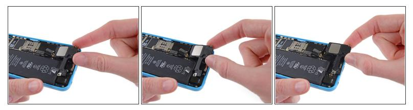
• Remove the speaker enclosure. Be careful not to snag it on the antenna cable.
