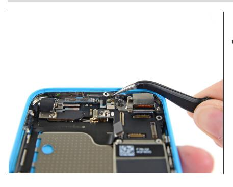
Use tweezers to remove the logic board grounding clip.
