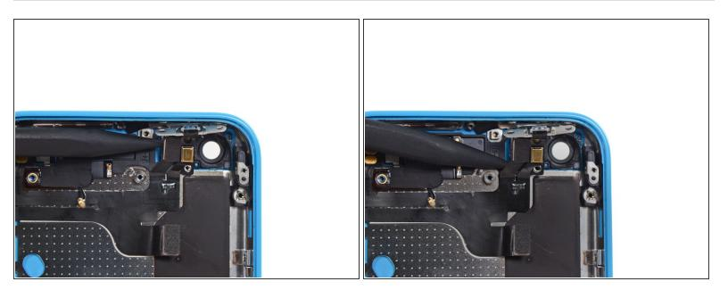
Run a spudger gently under the flash assembly cable to separate it from the phone.
