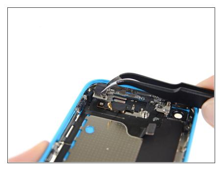
Remove the vibrator motor.
