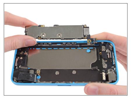
Remove the logic board from the rear case.
