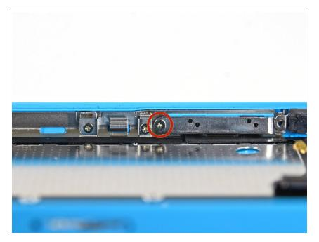
Remove the 1.6 mm Phillips #000 screw securing the volume rocker bracket to the side wall.
