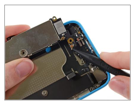
Disconnect the antenna connector from the back of the logic board.
