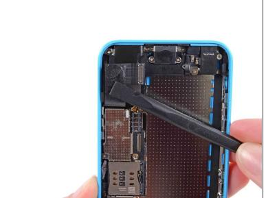
Flip the Lightning connector cable up out of the way of the logic board.
