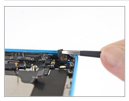
Remove any foam tape obscuring the screws near the camera cavity.
