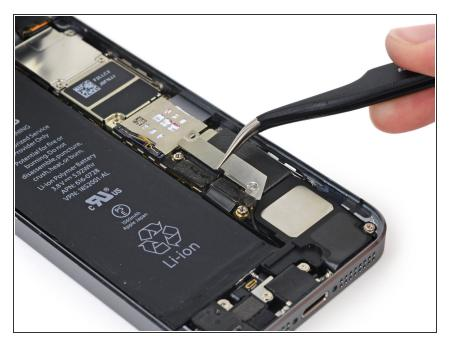
Remove the metal battery connector bracket from the iPhone.
