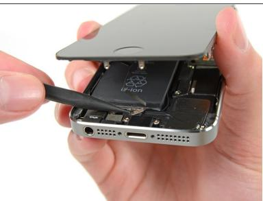
Use the tip of a spudger to pry the home button cable connector up out of its socket.
