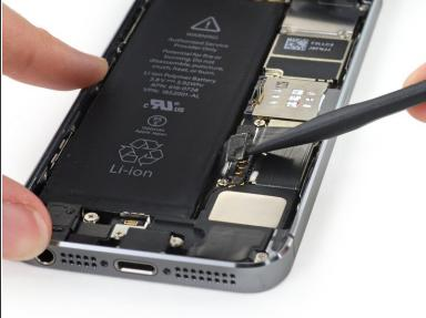
Use the flat end of a spudger to gently pry the battery connector up from its socket on the logic board.
