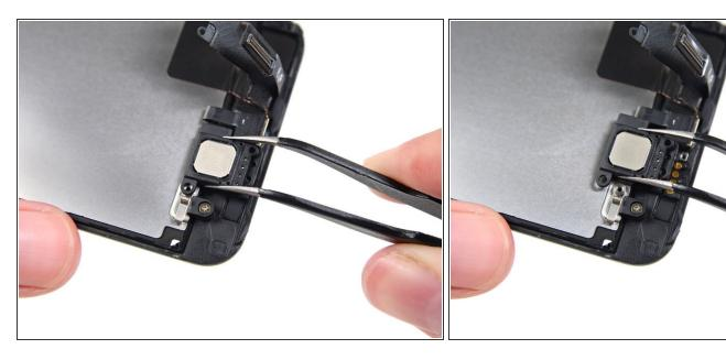
Remove the earpiece speaker with a set of tweezers.
