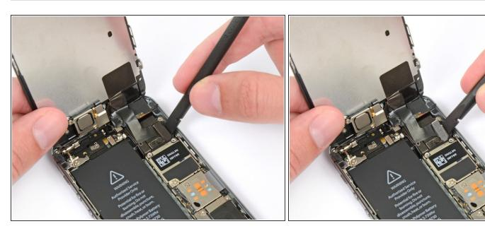
Use the flat end of a spudger to disconnect the front-facing camera and sensor cable.
