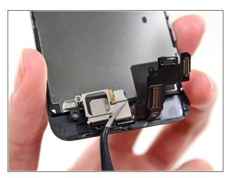
Remove the bracket from the display.
