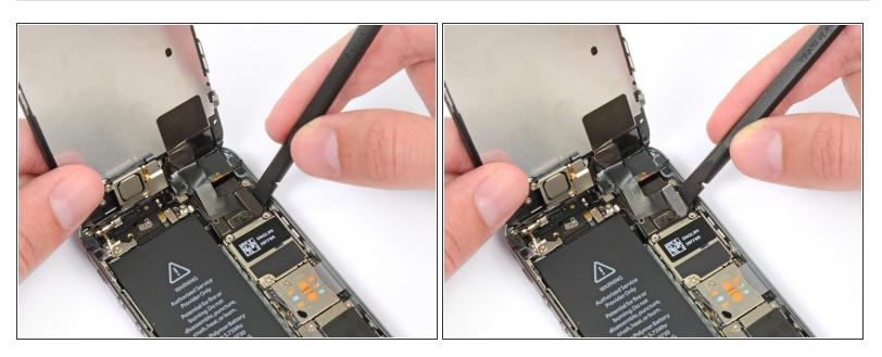
• Use the flat end of a spudger to disconnect the front-facing camera and sensor cable.
