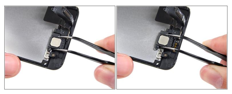
• Remove the earpiece speaker with a set of tweezers.
