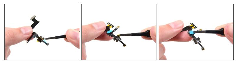
• Remove any clear backing strips from the light sensor, cable and front-facing camera.
