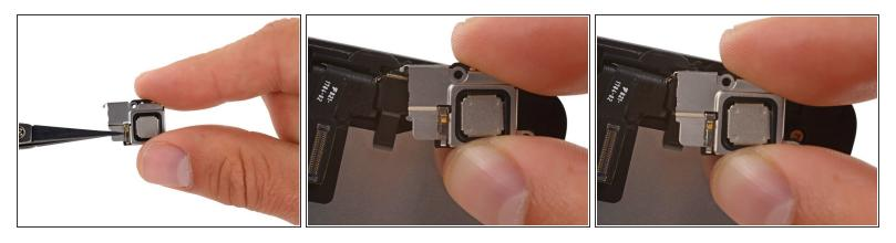
To replace the earpiece speaker, it is easiest to install the speaker and bracket together:
