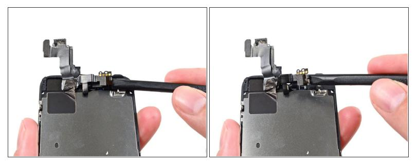
Use the flat end of a spudger to gently peel the front-facing camera portion of the cable away from the display assembly.
