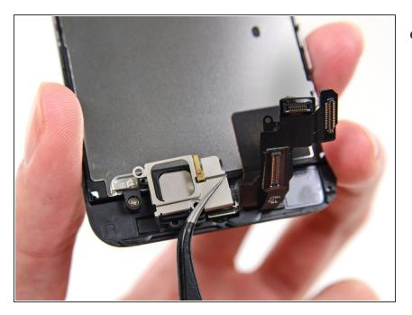
Remove the bracket from the display.
