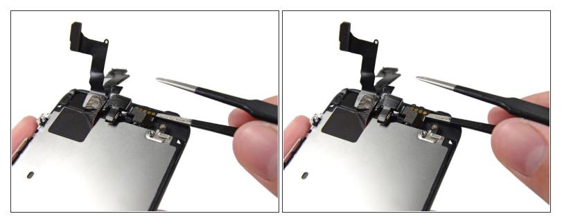
• Using the edge of a set of tweezers or a metal spudger, gently pry the earpiece speaker contact cable up, to separate this portion of the camera and sensor cable from the adhesive below.
