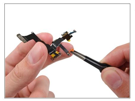
Remove any plastic coverings from the microphone on the sensor cable assembly.
