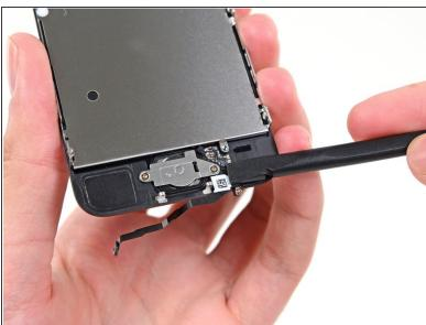
Fold the home button cable down, out of the way of the home button bracket.
