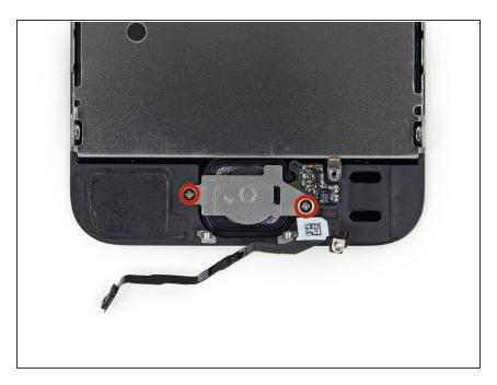
Remove the two 1.4 mm Phillips #000 screws from the home button bracket.
