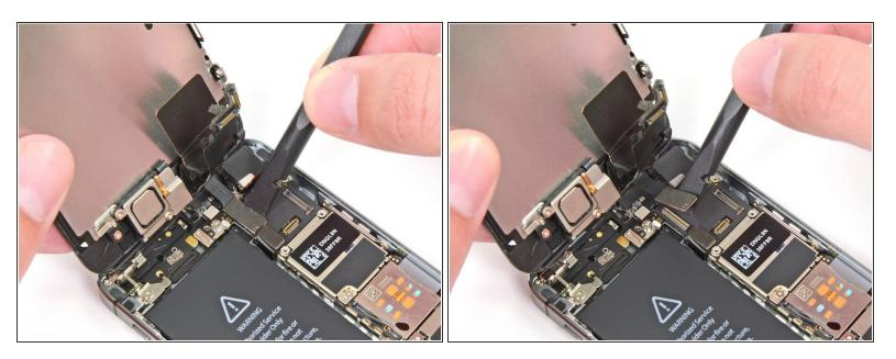
• Finally, disconnect the digitizer cable connector.
