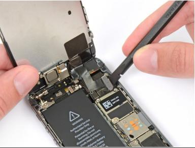
• Use the flat end of a spudger to disconnect the front-facing camera and sensor cable.
