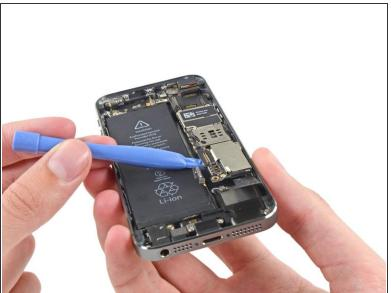
Use a plastic opening tool to lift the logic board up enough to grab with your fingers.
