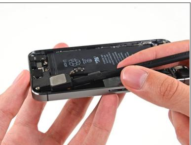
Use the flat end of a spudger to gently lift the speaker from the rear case.
