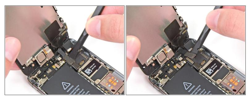
• Finally, disconnect the digitizer cable connector.
