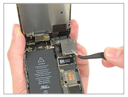
• Remove the front panel assembly cable bracket from the logic board.
