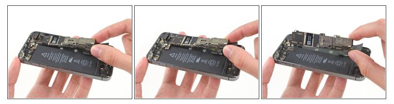
• Pull the logic board slightly away from the rear facing camera.
