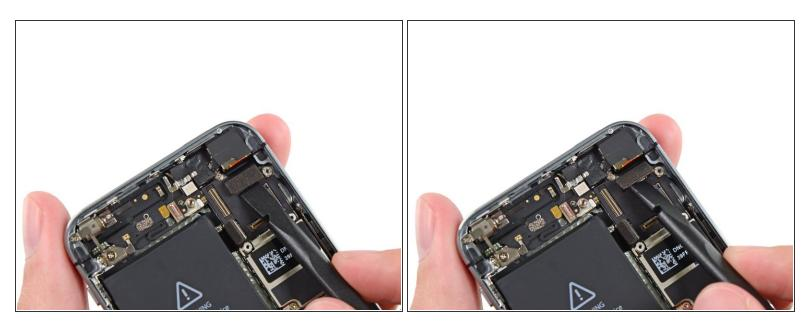
Use the flat end of a spudger to disconnect the rear-facing camera cable from its socket on the logic board.
