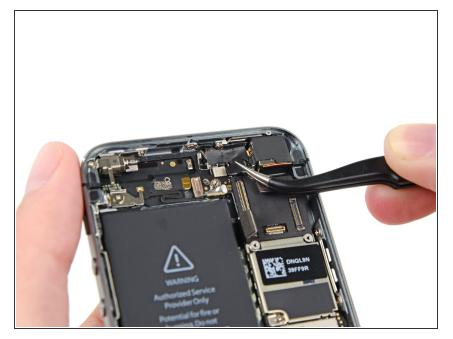
• Remove any tape covering the camera flash bracket.
