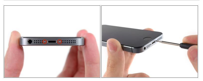
Remove the two 3.9 mm Pentalobe screws next to the Lightning connector.
