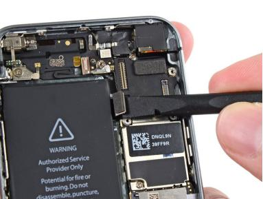
Use a spudger to gently pry the button assembly cable up from its socket on the logic board.
