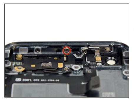
Remove the 1.3 mm Phillips #000 screw securing the logic board grounding bracket to the rear case.
