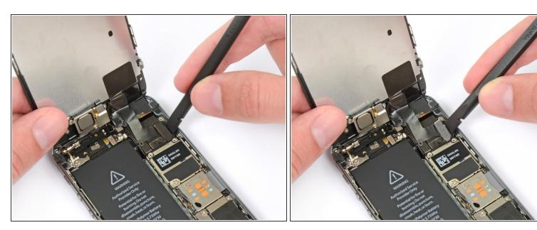
• Use the flat end of a spudger to disconnect the front-facing camera and sensor cable.
