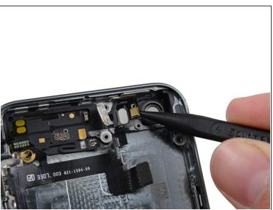
Use the tip of a spudger to free the microphone portion of the assembly from the case.
