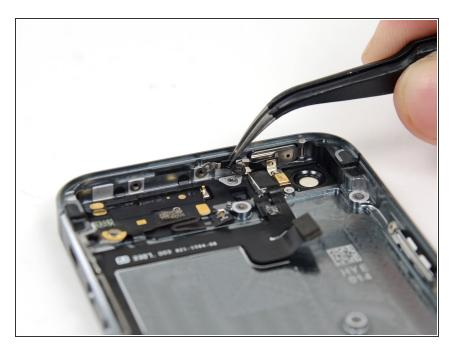
Remove the logic board grounding bracket.
