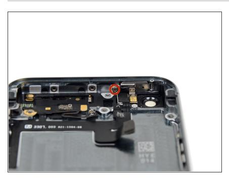
Remove the 2.1 mm Phillips #000 screw securing the contact clip and power/sleep button bracket.
