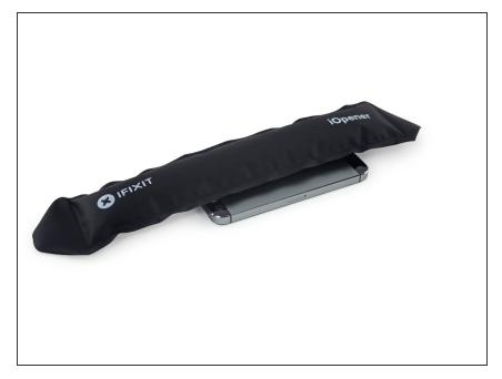
If any of the adhesive strips broke off and the battery remains stuck to the rear case, [invalid guide link] or use a hair dryer to heat the rear case directly behind the battery.
