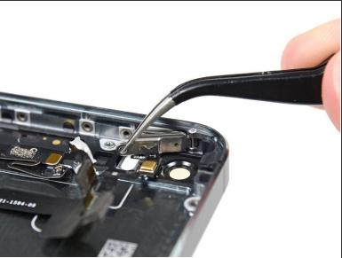
Use a set of tweezers to swing the power/sleep button bracket away from the case.
