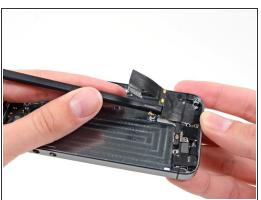
Slide the flat end of a spudger under the right-hand side of the lightning connector cable assembly to free it from the rear case.
