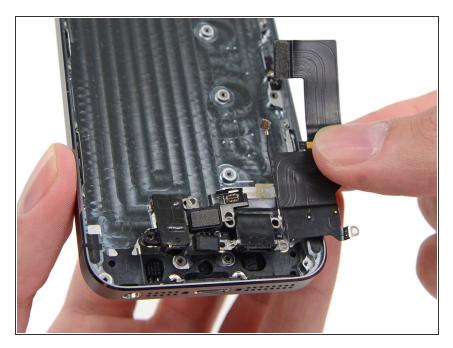
Remove the lightning cable assembly from the rear case.
