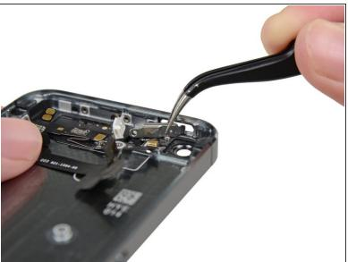
Unclip the power/sleep button bracket hinge from the post holding it in the iPhone.
