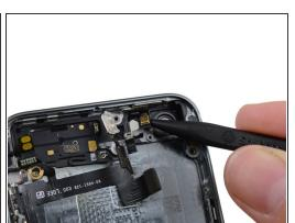
• Use the tip of a spudger to free the microphone portion of the assembly from the case.
