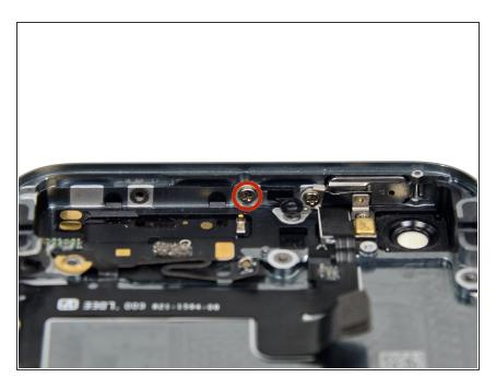
Remove the 1.3 mm Phillips #000 screw securing the logic board antenna bracket to the rear case.
