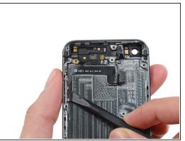
Run the flat end of the spudger under the portion of the cable near the volume control buttons.
