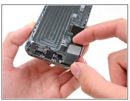
Remove the speaker by lifting it up and out of the rear case.
