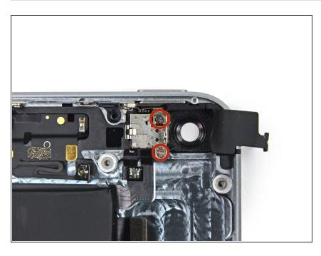
Remove the two 1.6 mm Phillips #000 screws securing the rearfacing camera bracket.
