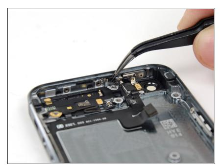
Remove the logic board antenna bracket.
