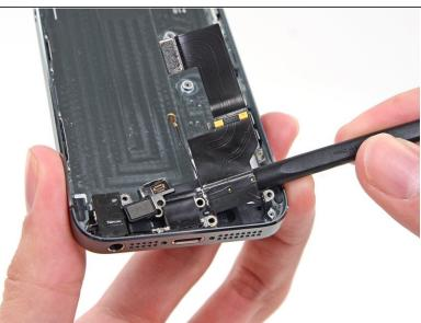
Continue to detach the lightning cable assembly by sliding the spudger under the port components.
