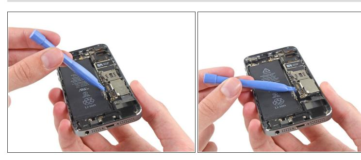
Use a plastic opening tool to lift the logic board up enough to grab with your fingers.
