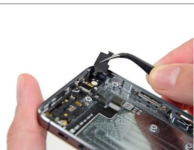
Use tweezers to pull the rubber rear-facing camera cover out of its slot in the rear case.
