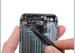
Slide the flat end of a spudger under the upper component assembly cable to free it from the rear case.
